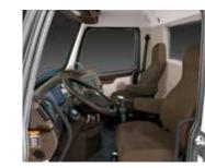
Easy in and out. Doors are 3+ feet wide and open a full 70 degrees for ease of access. Ergonomically placed grab handles provide the safest and most secure way in and way out of the cab.
