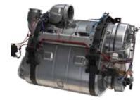
One-box aftertreatment. Volvo's "one-box" exhaust aftertreatment system offers smaller system packaging and reduces weight by 17 pounds compared to current systems. The one-box configuration provides better thermal encasing of exhaust energy, and improves muffler efficiency. The use of Cu-Z (copper zeolite) catalyst coatings improves both low-temperature NOx conversion, and long-term system robustness.
