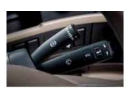
The intelligent Volvo Engine Brake (VEB) is an enhanced engine braking system that gives drivers precise control over engine braking, and saves the truck's brakes for when they're needed most. The D11 and D13 engines use a Variable Geometry Turbocharger (VGT), which, thanks to intelligent software, "supercharges" the VEB system. The result is phenomenal retarding horsepower at low rpm, where the engine spends most of its time and where braking is needed most.
