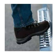
Secure access. At Volvo, driver safety begins even before the engine starts. Self-cleaning steps ensure secure footing during cab ingress and egress, while ergonomic grab-handles provide a solid grip, even when wearing gloves.
